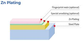
Various post-processing functions available, such as non-treatment, coating, phosphate, anti-fingerprint, and black resin are available, and are mainly used for home appliances.
