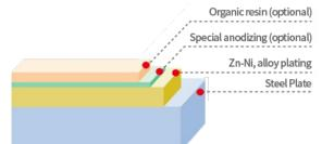
Possible to select oil, phosphate, functional resin (fuel tank), etc. and be mainly used for automobiles.
